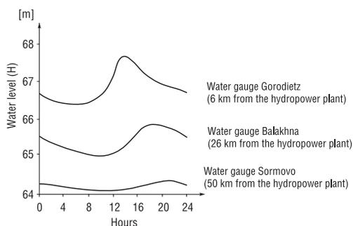
Figure 1. Diurnal water level fluctuation pattern on the Nizhny Novgorod hydropower dam tailwater on the River Volga
