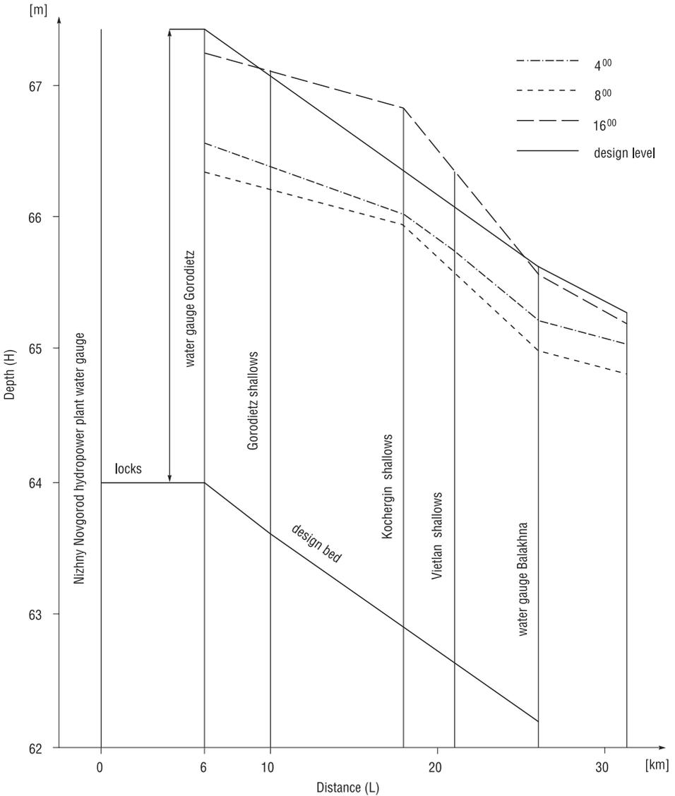
Figure 2. Free water levels at the average mean daily discharge of  $1100 \text{ m}^3\cdot\text{s}^{-1}$  (30 September 1999)
