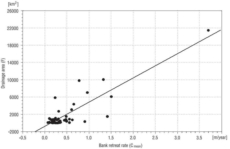
Figure 9. Annual average bank retreat rate ( $C_{mean}$ ) versus drainage area ( $F$ )
