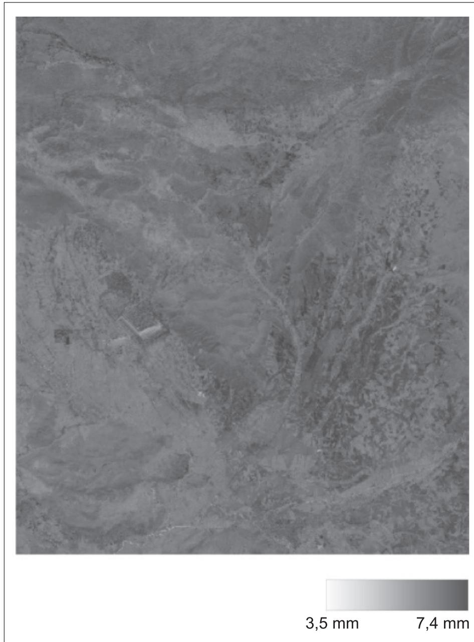
Figure 2. Evaporation values of the basin, dark parts are heavily evaporated rather than white parts, (ASTER July, 6, 2006)
