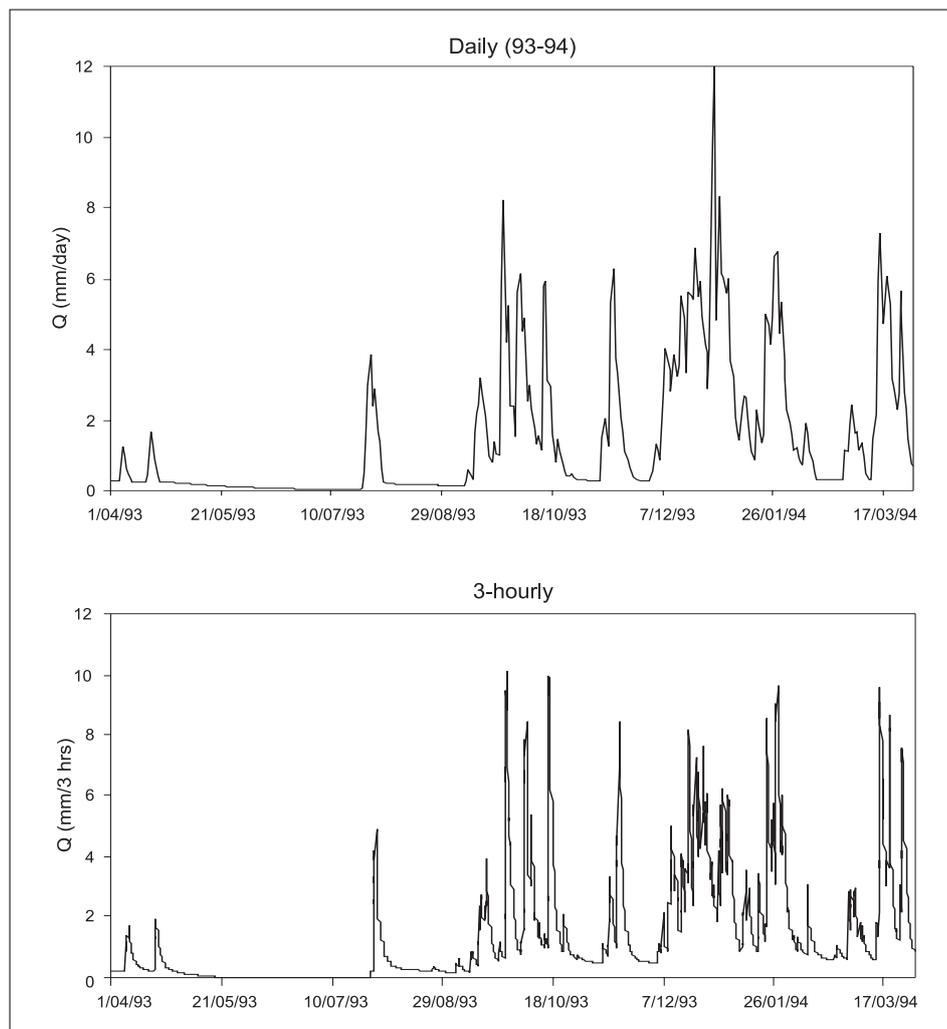
Figure 2. Computed outflow of Hupsel for the year 93-94 at daily ( $\text{mm}\cdot\text{d}^{-1}$ ) and 3-hourly ( $\text{mm}\cdot 3\text{h}^{-1}$ ) time steps
