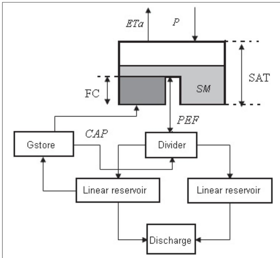
Figure 1. The structure of the Wageningen Rainfall runoff model
