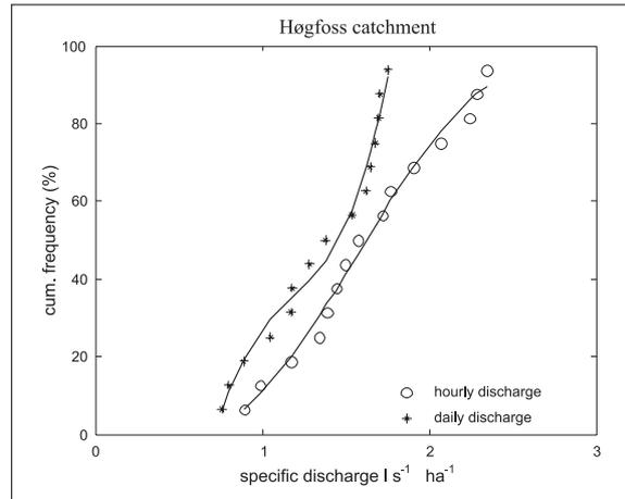
Figure 2. Specific discharge for Høgfoss based on hourly and average daily discharge values
