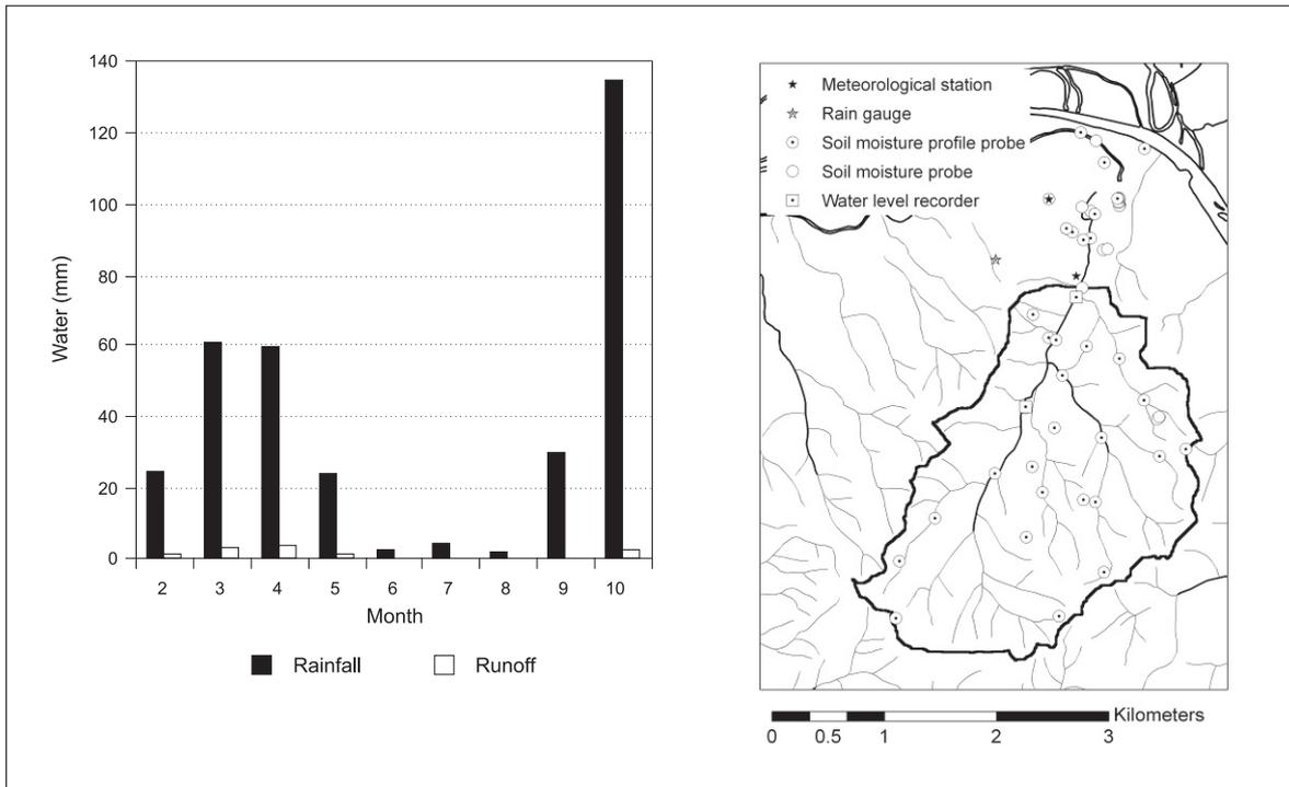
Figure 2. Monthly water balance in the Covões catchment for 2005, during the monitoring period (left). Map of current and future monitoring equipment (right)
