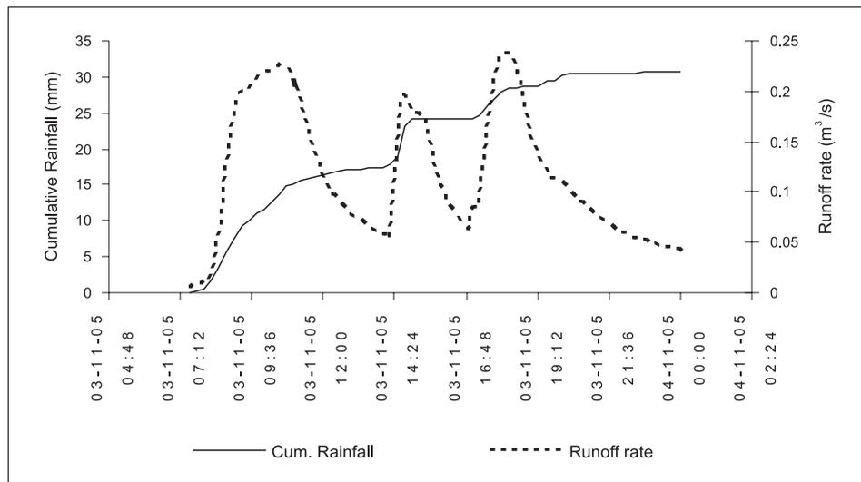
Figure 3. Cumulative rainfall and corresponding hydrograph for a selected storm
