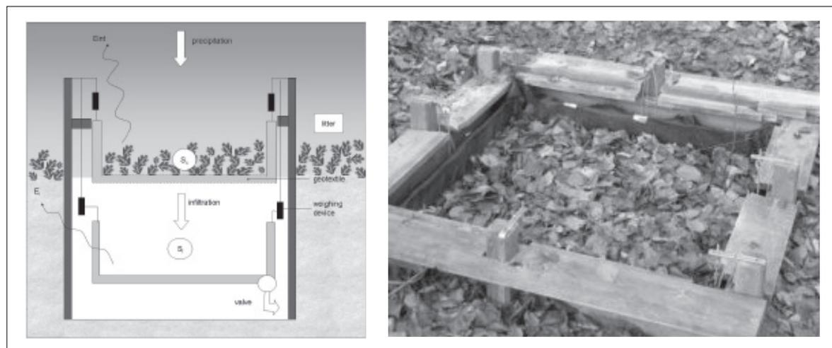
Figure 2. Schematic drawing (left) and picture of the forest floor device in the Huewelerbach catchment (right)
