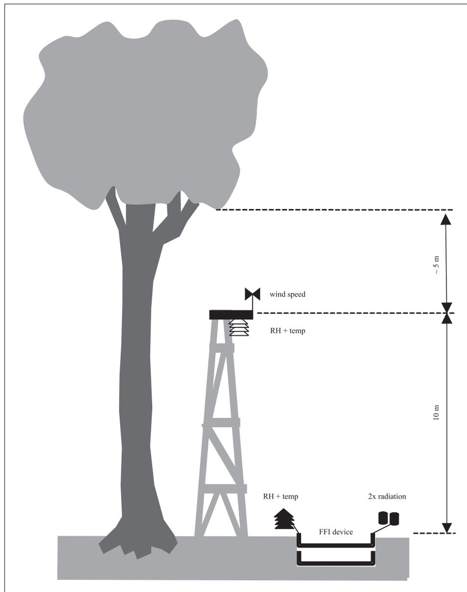
Figure 3. Overview of the measuring setup for the energy balance model (RH = relative humidity sensor; temp = temperature sensor; FFI device = forest floor interception device)
