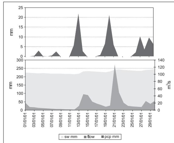
Figure 1. Measured daily rainfall flow and simulated daily discharge and mean soil water content
