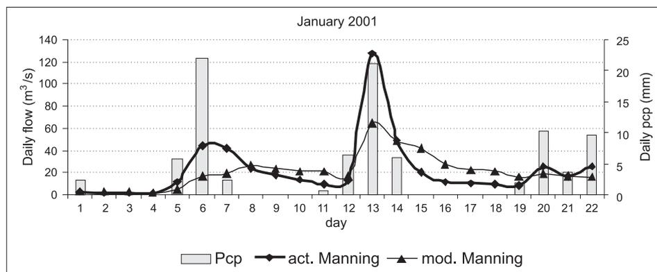
Figure 2. Simulated flow (actual and the modified Manning's coefficient)
