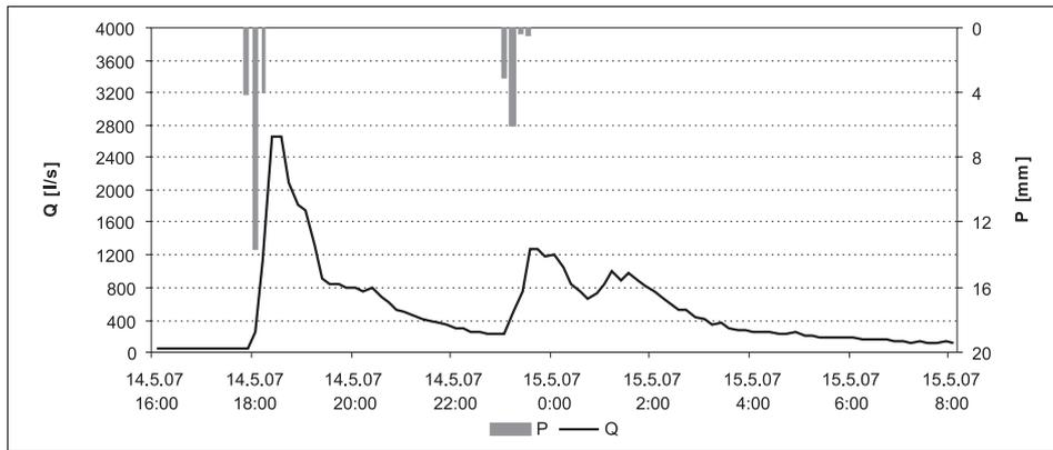
Figure 1. Precipitation and discharge during the heavy rain event May 14th/15th 2007 (first event 21.7 mm, second one 10.0 mm)
