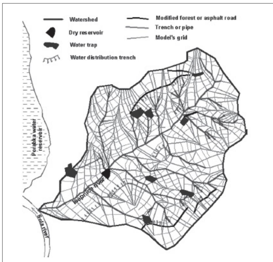
Figure 3. The Isepnica Torrent catchment with computation net and proposed SlowDown structures.
