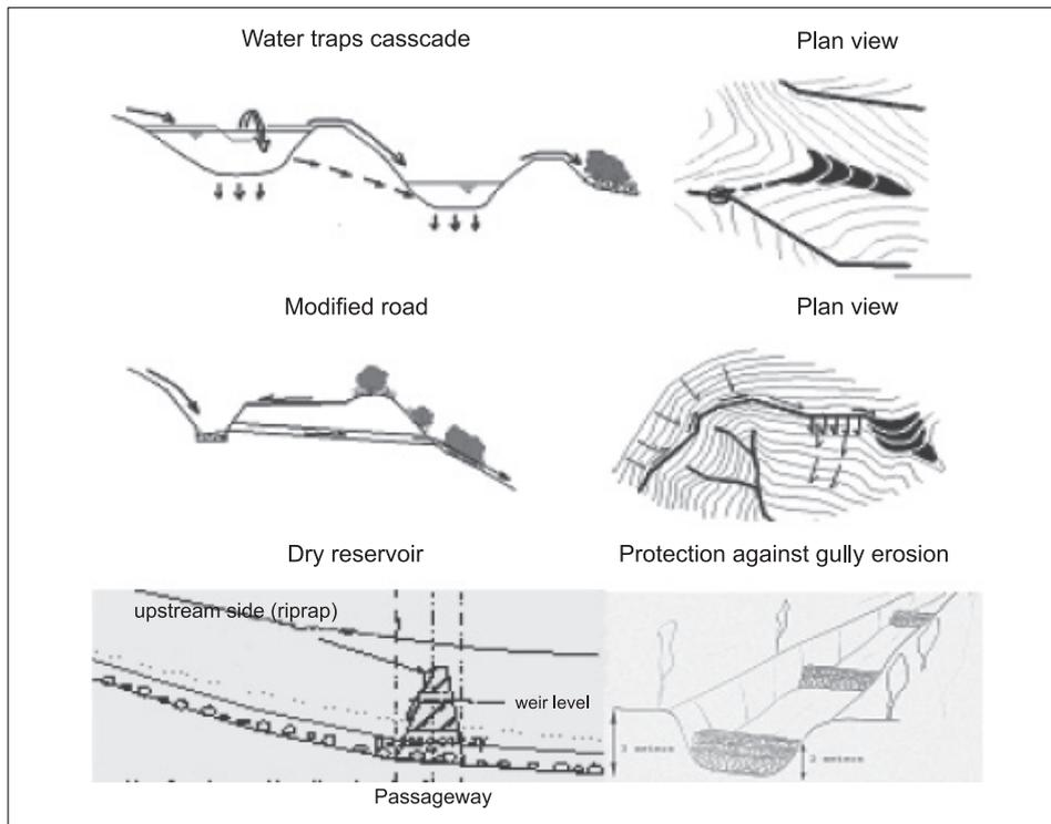
Figure 1. DSD catchment structures
