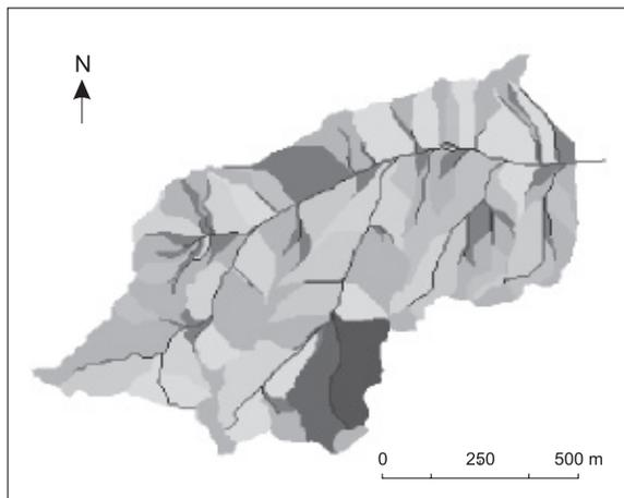
Figure 1. Layout of Ganspoel watershed discretisation in sub-watersheds and channels by GeoWEPP
