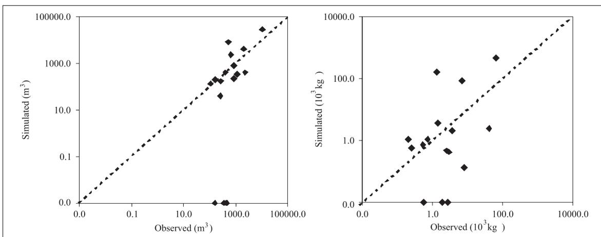
Figure 2. Comparison between observed and simulated runoff (left) and sediment yield events (right) for WEPP implementation in the Ganspoel watershed (simulation series *III*:  $K_e = 0.5\% K_{sat}$ )
