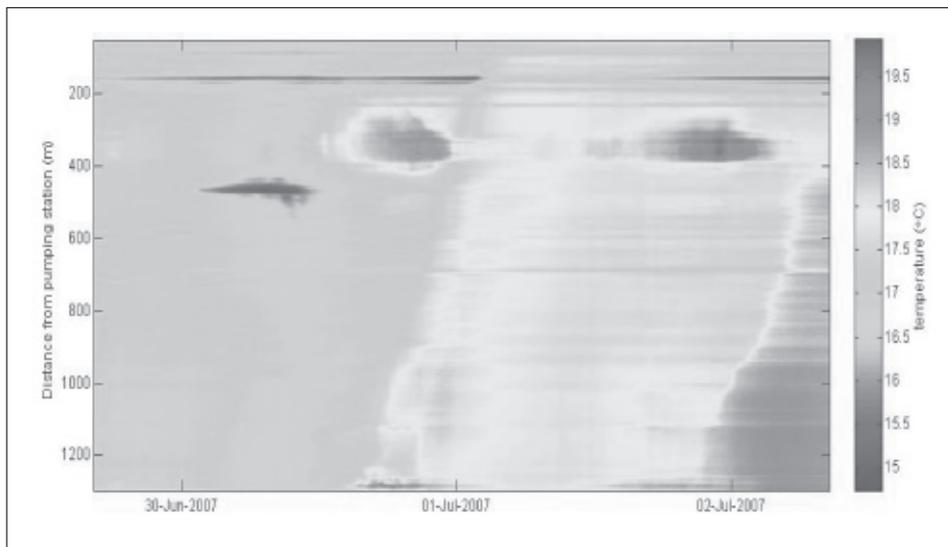
Figure 1. Example of the total ensemble of temperature effects along a 1300 meter cable in a canal in the Wieringermeerpolder
