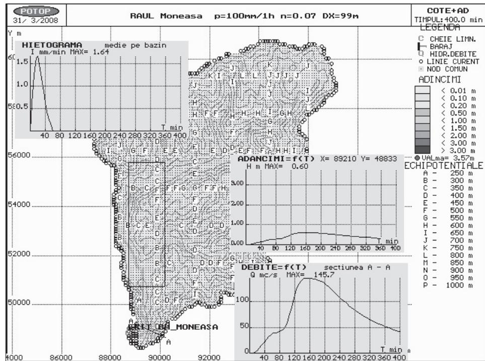
Figure 2. Simulation results for 100 mm rainfall and 0.07 mean roughness coefficient
