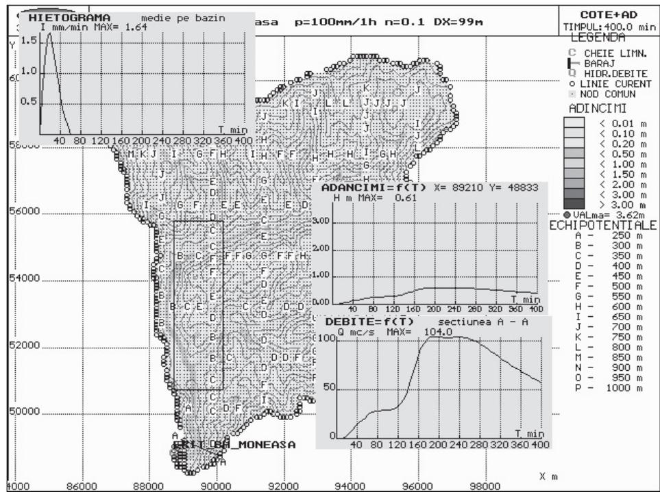
Figure 1. Simulation results for 100 mm rainfall and 0.1 mean roughness coefficient
