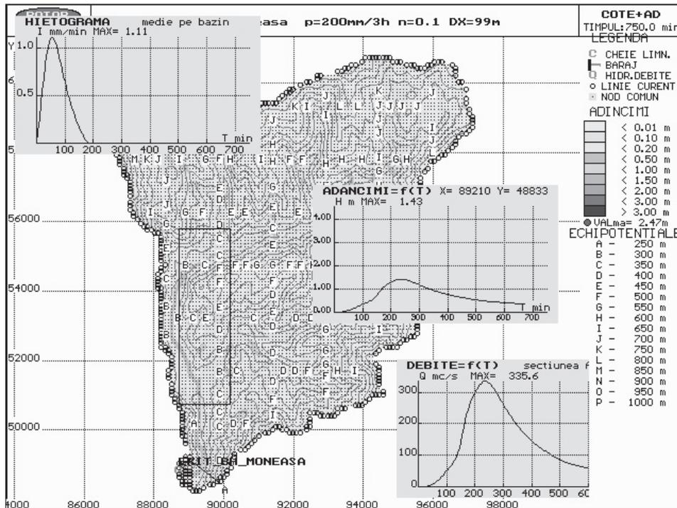
Figure 4. Simulation results for 200 mm rainfall, 3 hours duration and 0.1 mean roughness
