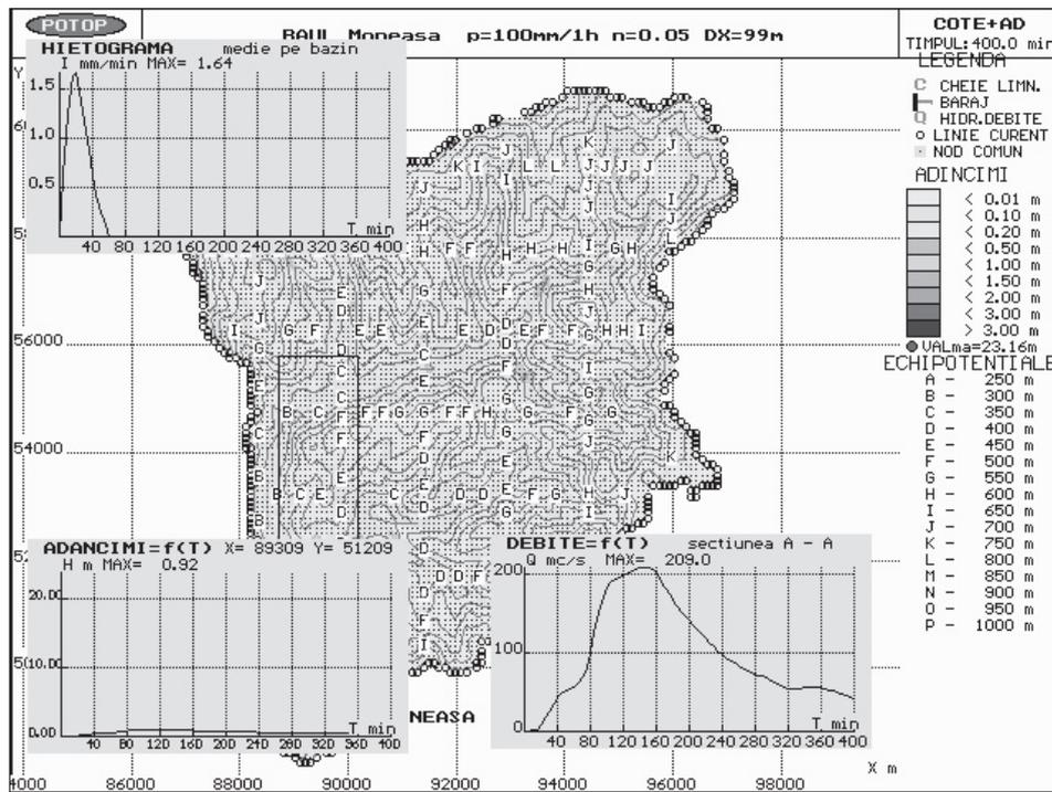
Figure 3. Simulation results for 100 mm rainfall and 0.05 mean roughness coefficient
