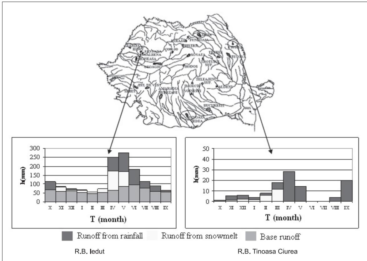
Figure 1. The water runoff mean monthly values from the characteristic years: 1975 in the R.B.Iedut case and 1981 in the R.B. Tinoasa Ciurea case
