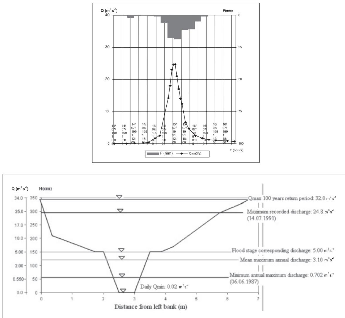
Figure 3. The largest flood recorded (14.07.1991) and characteristic thresholds of the maximum discharges in the section of the hydrometric station – Iedut river
