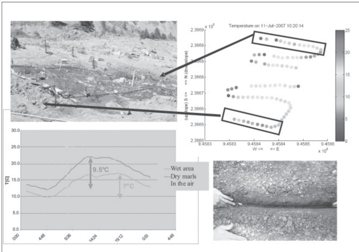
Figure 2. Example of DTS measurements analyses
