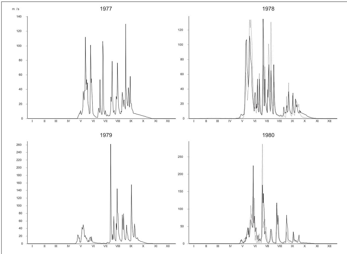
Figure 2. Observed (solid line) versus simulated (dotted line) hydrographs, Timpton at Nagorniy,  $F = 613 \text{ km}^2$ , 1977-1980
