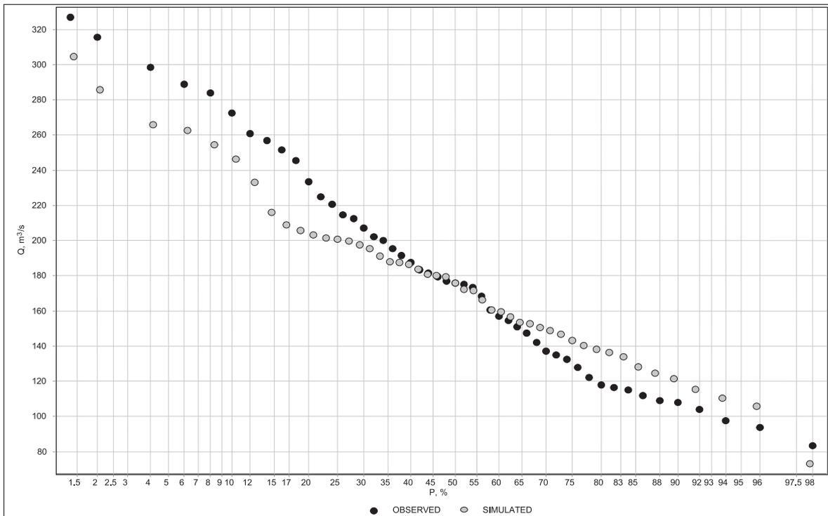
Figure 3. Observed versus simulated empirical distribution curves of maximum floods, Timpton at Nagorniy,  $F = 613 \text{ km}^2$
