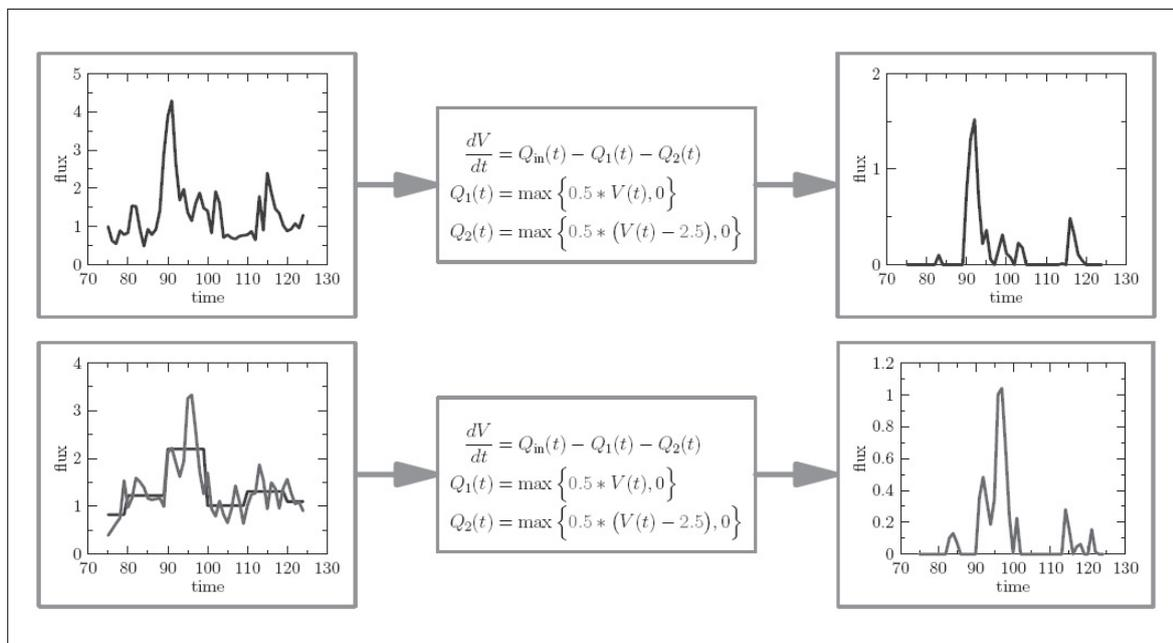
Figure 2. At the top the available knowledge is shown. At the bottom left, the available low resolution input means are stochastically disaggregated into high resolution input and can as such be used for existing model to produce high resolution output. This procedure should be used in a Monte-Carlo framework: many inputs should be simulated and the corresponding outputs should be analyzed statistically
