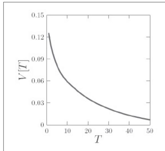
Figure 3. A typical variation reduction function, showing how the variation in time series diminishes as one averages out over large time intervals
