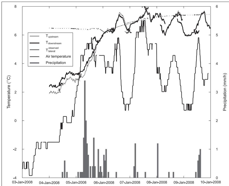
Figure 2. The temperature of lateral inflow first cools down after a rain event, before it warms up by about 1.5 °C
