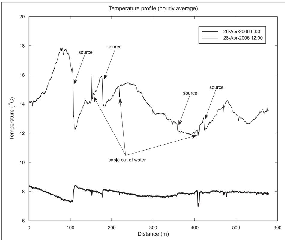
Figure 1. Longitudinal temperature profile of the Maisbich. Thick line is at 06:00, the thin line at 12:00 of the same day
