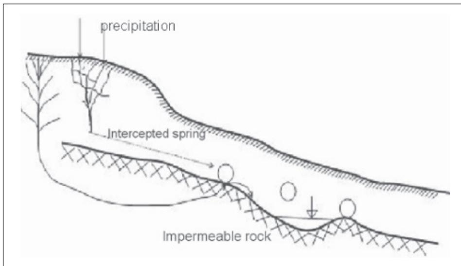
Figure 3. Tile drainage runoff formation by springs
