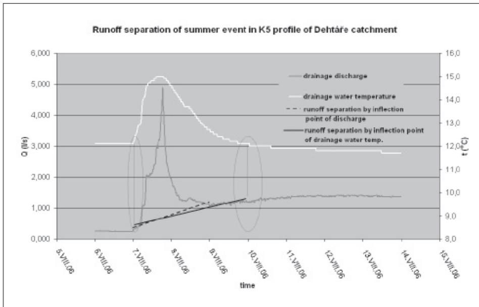
Figure 2. Attempt to fast runoff component separation by changed drainage water temperature
